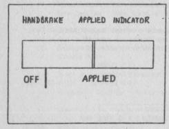
WHENEVER POINTER IS ANYWHERE IN THE 'APPLIED' SECTOR - BEFORE MOVEMENT IS UNDERTAKEN; WIND HANDWHEEL ANTI-CLOCKWISE ONTO STOP UNTIL POINTER IS IN THE 'OFF' SECTOR.
