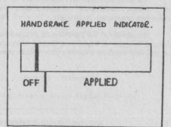
WHENEVER POINTER IS IN 'OFF' SECTOR -HANDBRAKE IS RELEASED: TO APPLY -WIND HANDBRAKE WHEEL CLOCKWISE UNTIL IT IS SOLID AND NOT ONLY UNTIL POINTER REACHES 'APPLIED' SECTOR.
